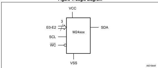
Figure 1. Logic diagram
