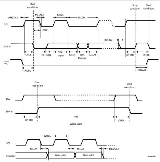
Figure 16. AC waveforms
