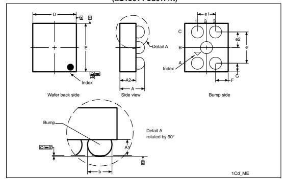
Figure 22. WLCSP 5-bump wafer-length chip-scale package outline (M24C64-FCS6TP/K)
