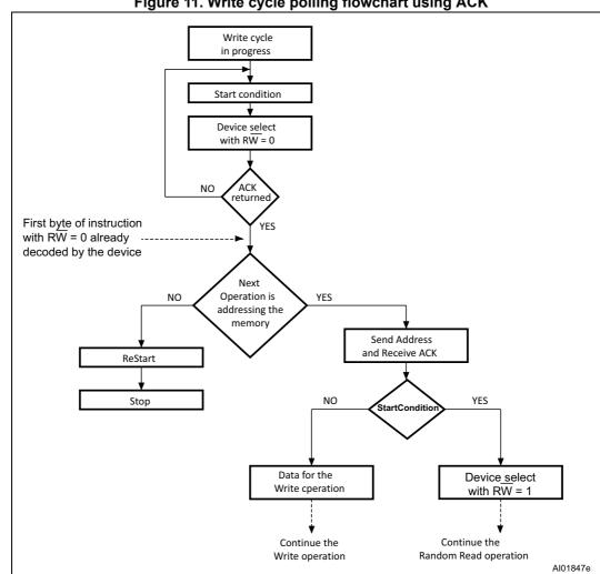
Figure 11. Write cycle polling flowchart using ACK
