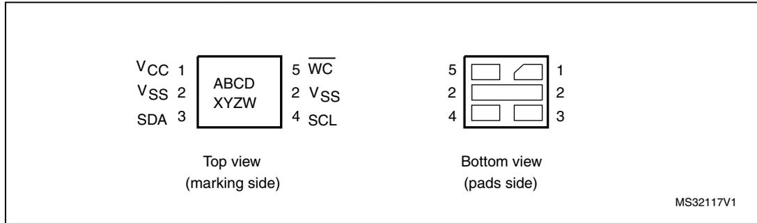
*Note:* Inputs E2, E1, E0 are not connected, therefore read as (000). Please refer to [Section 2.3](#) for further explanations.
