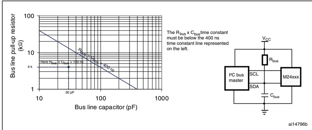
Figure 15. Maximum  $R_{bus}$  value versus bus parasitic capacitance ( $C_{bus}$ ) for an I<sup>2</sup>C bus at maximum frequency  $f_C = 1$  MHz
