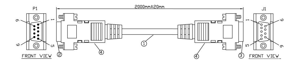
1.CABLE:NO UL.,28AWG(7/0.12±0.008mm),TINNED AND STRANDED COPPER WIRE INSULATOR:PVC,ID:0.85mm ,CABLING:9C+DRAIN WIRE
